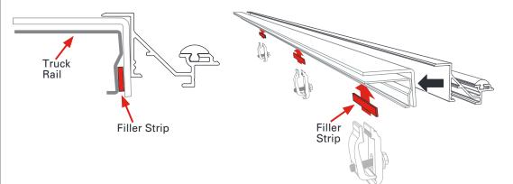
IMPORTANT: In order for the cover (C) to operate properly the side rails (A & B) MUST be square (90° angle) to the truck bed rails. This allows the rear latch to engage properly.
