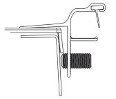
If the rails measured too close together, turn the screws counter clockwise.
